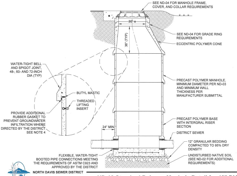
ND-12 Standard Polymer Manhole Detail for 42" DIA Sewer or Smaller 1 of 3
